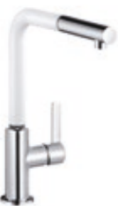
single lever sink mixer DN 15 swivelling spout, pull-out hand spray H1 295, H2 265, A 220, Ø2 38 408519375 □
